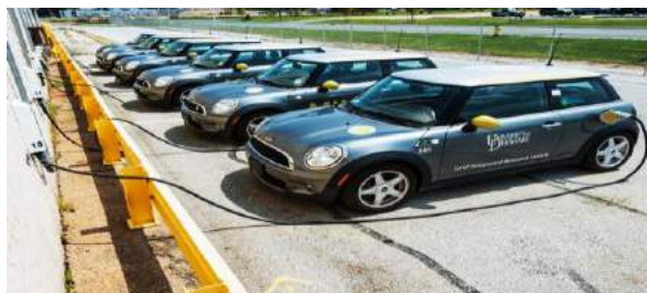
Figure 5.12: University of Delaware's V2G system
